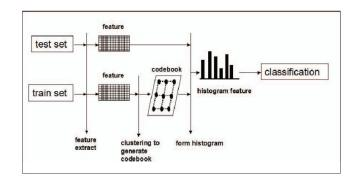
Fig. 1. The structure of proposed BoW model
