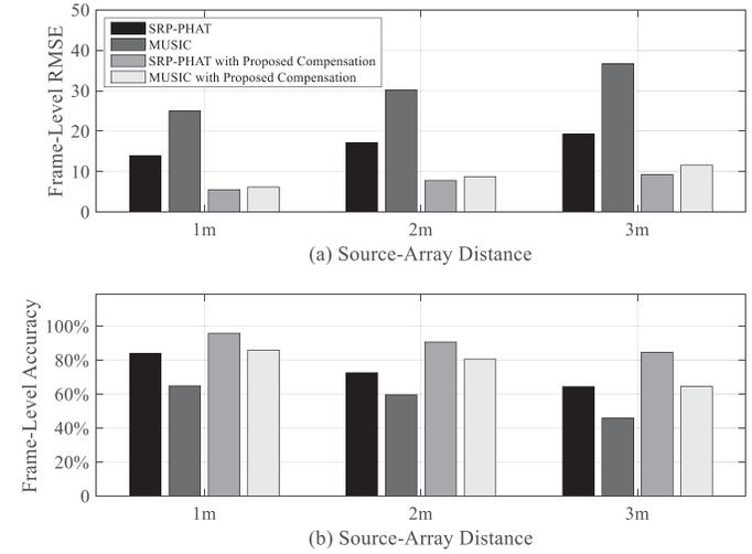
Fig. 4. Frame-level RMSE (a) and Accuracy (b) of different algorithms using uniform circular array (UCA) for different source-array distances.
