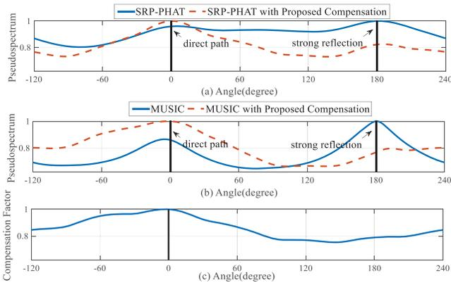
Fig. 3. The pseudo spectrum of SRP-PHAT and compensated SRP-PHAT (a), the pseudo spectrum MUSIC and compensated MUSIC (b), corresponding compensation factor (c). Direct-path DOA angle is 0 marked with vertical solid line. Reflection-path DOA angle is 180 marked with vertical dotted line. Reverberant environment: T60 is 600ms + 20dB SNR white Gaussian noise + uniform circular array (UCA) closet to a strong reflector.
