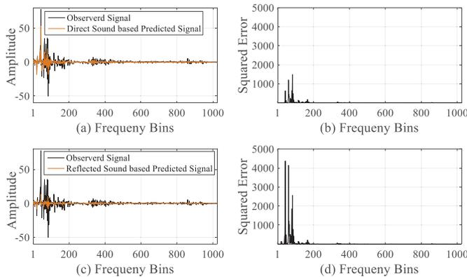
Fig. 2. The frequency-domain presentation of observed signal, signal predicted using the beamformed signal from the source (a) and reflection (c). (b) and (d) represent corresponding squared error of (a) and (c), respectively.
