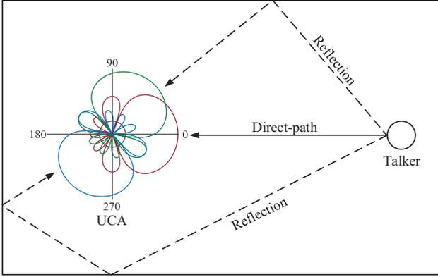
Fig. 1. Schematic illustration of uniform circular array (UCA) based beamforming towards different hypothesized DOAs.
