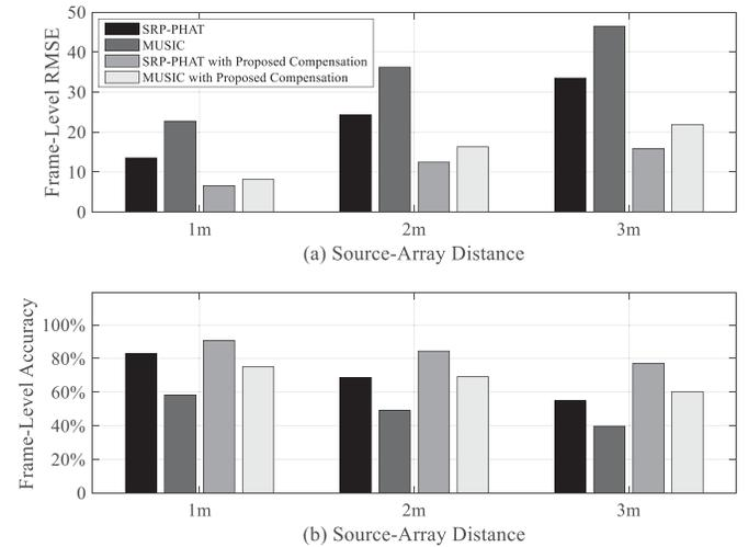
Fig. 5. Frame-level RMSE (a) and Accuracy (b) of different algorithms using dual-microphone array for different source-array distances.
